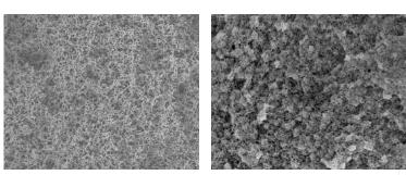
SEMs of TIPS(Left) and NIPS (right) surfaces, demonstrating the strong multiple crosslinks of the TIPS fiber.
